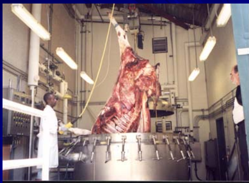
Loading partial bovine carcass into the Tissue Digester
