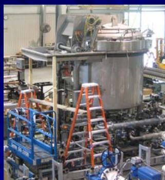
5,000 lb Capacity CDU for Cornell CVM in PRI Plant
