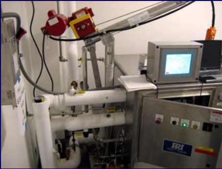
All External Piping is Safety Insulated
