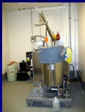
Tufts CDU With Safety Insulation Jacket Over Lid
